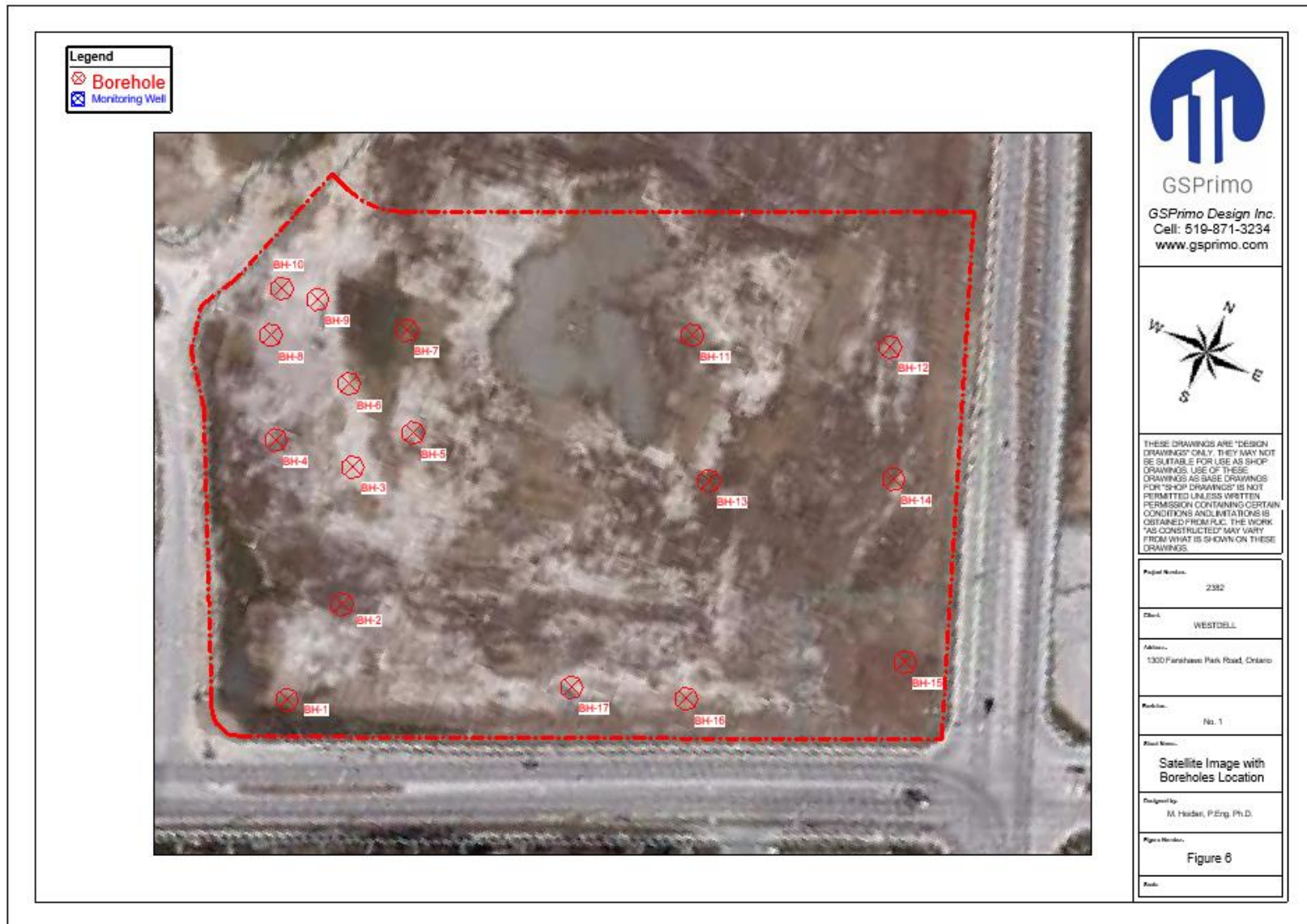
Figure 6 – Geotechnical boreholes location, Site Plan
